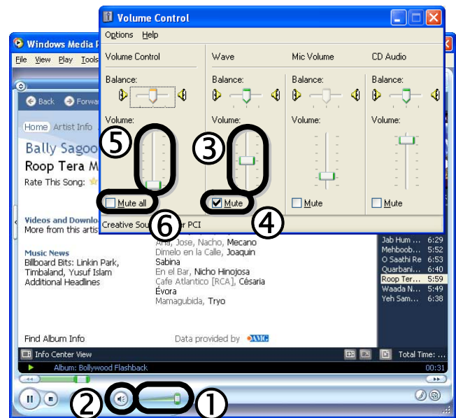
Figure 1: Current volume control model: application audio output is only active when its volume slider (1) and wave and master sliders in the control panel (3, 5) are set to non-zero values and the three mute check boxes (2, 4, 6) are unchecked.
